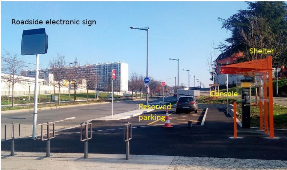
Fig. 5. Configuration of a physical meeting point for the 'Lane' carpooling service. The orange structure is like a bus shelter. A passenger notifies potential drivers of their carpooling request using the console, which is then displayed on the roadside electronic sign. A driver can safely embark the passenger in the reserved parking place. Reproduced with permission from Ecov.
